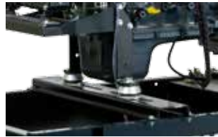
Heavy duty anti-vibration mountings
