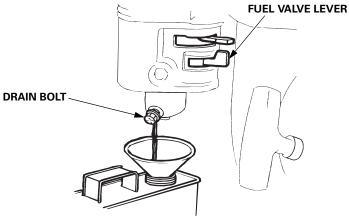
3. After all fuel has drained, tighten the carburetor drain bolt securely, move the fuel valve lever to the OFF position.
