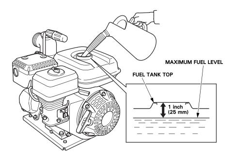
Refuel in a well-ventilated area before starting the engine. If the engine has been running, allow it to cool. Refuel carefully to avoid spilling fuel. Do not fill the fuel tank completely. Fill tank to approximately 1 inch (25 mm) below the top of the fuel tank to allow for fuel expansion. If may be necessary to lower the fuel level depending on operating conditions.
