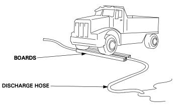
Driving over a discharge hose while the pump is running, or even possibly when the pump is stopped, may cause pump case failure.
