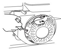
Align the notch on the pulley with the hole at the top of the cover.
