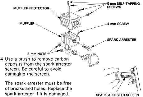
5. Install the spark arrester, muffler protector, and muffler in the reverse order of disassembly.
