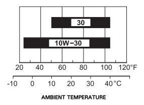
SAE 10W-30 is recommended for general use. Other viscosities shown in the chart may be used when the average temperature in your area is within the recommended range.
