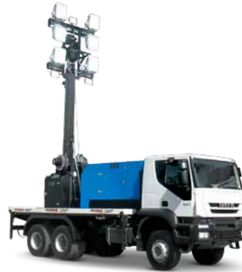
20 m lighting tower with 100 kVA generator on Iveco Maxi Truck
